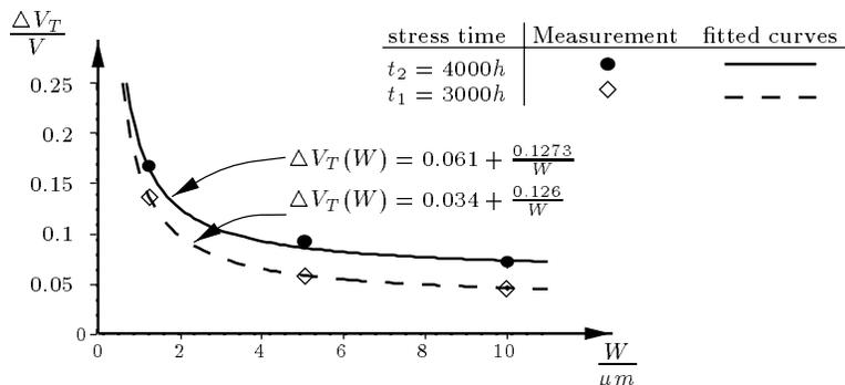
Figure 5:  $1/W$ -dependence of voltage shifts for fixed stress times  $t_1$  and  $t_2$  (see figure 4)
