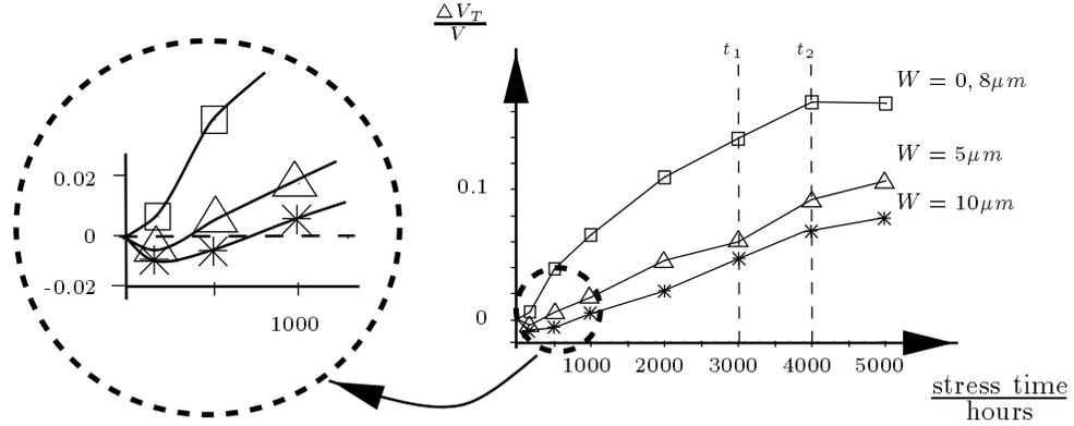
Figure 4: Stress time dependence of threshold voltage shift.
