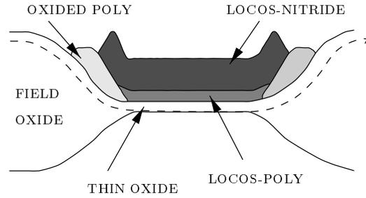
Figure 2: Cross-section from A to B (fig. 1) after the LOCOS Oxidation.
