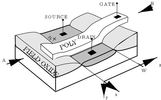
Figure 1: Typical structure of a MOSFET device.
