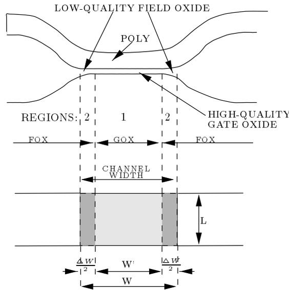
Figure 3: Cross-section from A to B (fig. 1) through the final transistor and top view illustrating the edge regions (regions 2) and the central region (region1).
