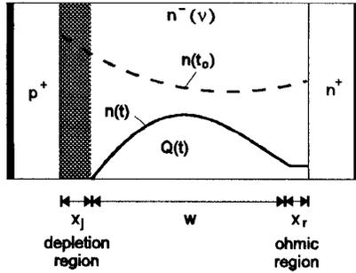
Figure 1: Structure of a p-v-n diode and charge carrier distribution in lightly-doped region during forward operation ( $n(t_o)$ ) and during turn-off ( $n(t)$ )
