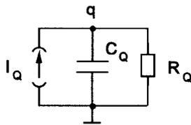
Figure 3: Subcircuit for stored charge
