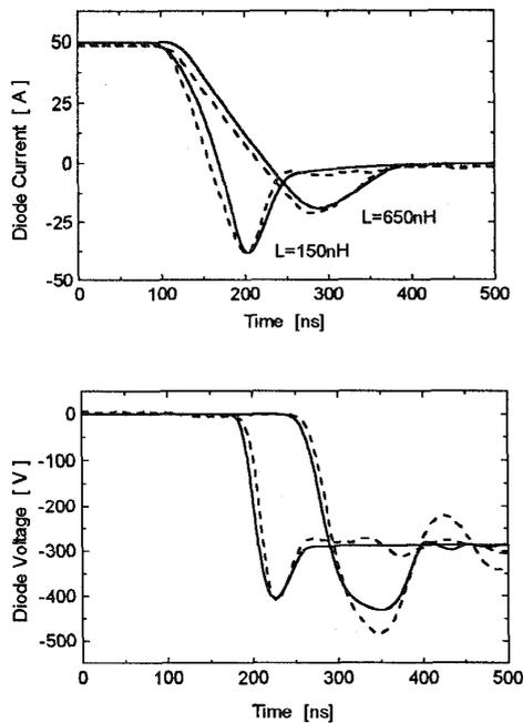
Figure 7: Reverse recovery of the power diode, comparison of simulations (—) and measurements (- -)
