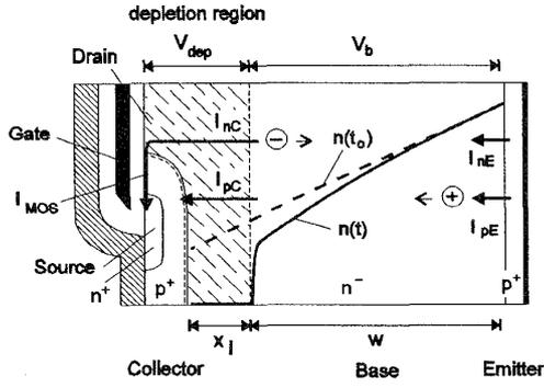
Figure 4: Structure of a NPT-IGBT and charge carrier distribution in base during stationary on-state ( $n(t_o)$ ) and during turn-off ( $n(t)$ )
