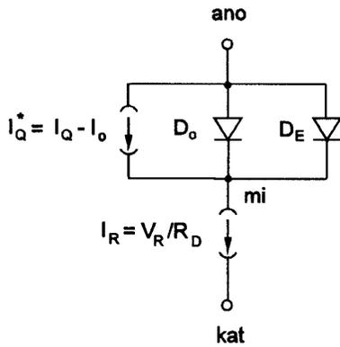
Figure 2: Subcircuit of the power diode
