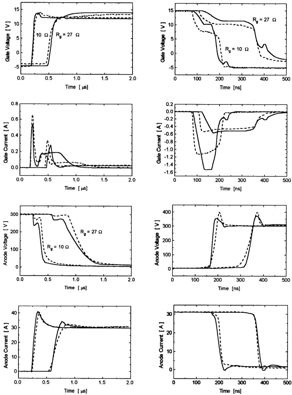
Figure 9: Turn-on (left column) and turn-off (right column) of an IGBT with inductive load and free-wheeling diode, comparison of simulations (—) and measurements (---)
