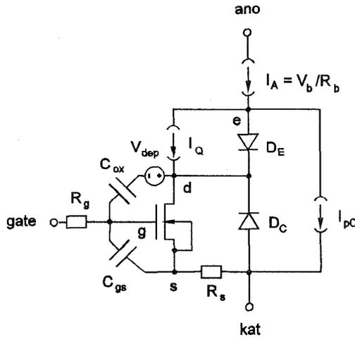
Figure 5: Subcircuit of the NPT-IGBT
