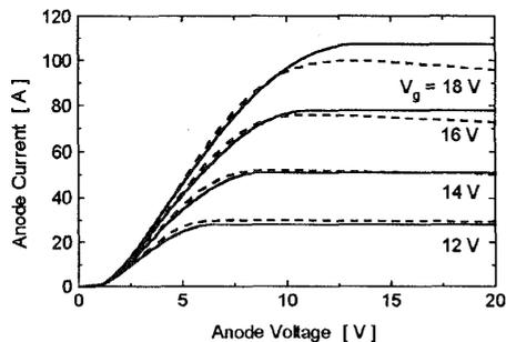
Figure 8: DC-characteristics of the IGBT, (—) simulations, (- -) measurements
