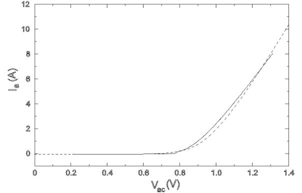
Fig. 13. Comparison between measurement (—) and simulation (- -) of DC-characteristic with manufacturer/fitted data.
