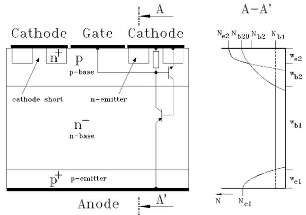
Fig. 1. Structure of a cathode-shortened SCR with equivalent circuit and doping profile.
