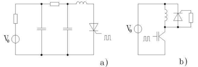
Fig. 5. Measuring circuits for passive (a) and active (b) commutation.
