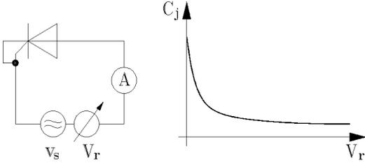
Fig. 2. Junction capacitance measurement.
