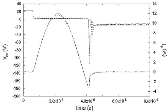
Fig. 11. Comparison between measurement (—) and simulation (- -) of passive commutation with manufacturer/fitted data.
