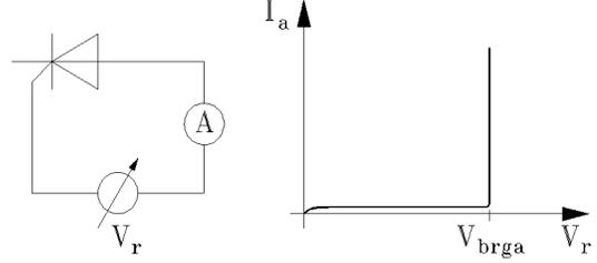
Fig. 3. Breakdown voltage measurement.
