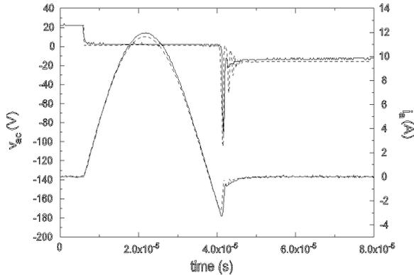
Fig. 12. Comparison between measurement (—) and simulation (- -) of passive commutation with extracted parameters.
