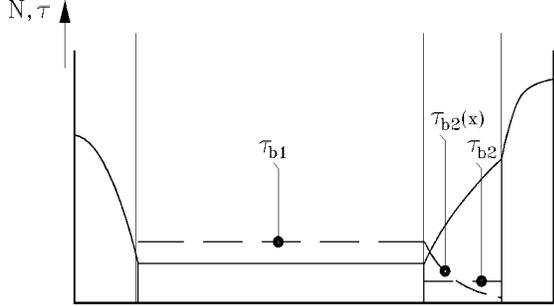
Fig. 8. Minority carrier lifetime in the  $n$ -base and the  $p$ -base.
