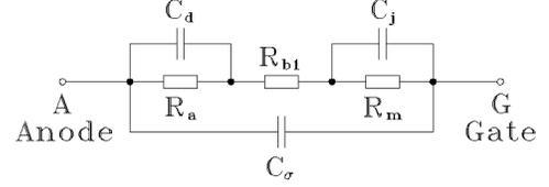
Fig. 7. Small signal model of the gate-anode structure ( $C_d$  diffusion capacity  $p^+n^-$ -junction,  $R_a$  differential resistance  $p^+n^-$ -junction,  $R_{b1}$   $n$ -base resistance,  $C_j$  junction capacity  $n^-p$ -junction,  $R_m$  differential resistance  $n^-p$ -junction,  $C_\sigma$  parasitic capacity).
