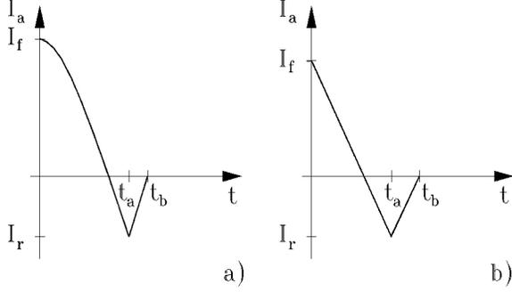
Fig. 6. Current waveforms for passive (a) and active (b) commutation.
