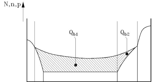
Fig. 4. Charge in the  $n$ -base and the  $p$ -base under static conditions ( $Q_{b1} \gg Q_{b2}$ ).
