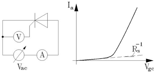
Fig. 9. Measuring the anode current as a function of gate-cathode voltage.
