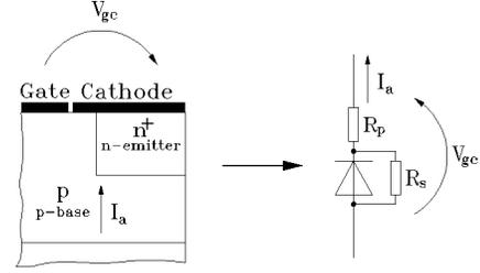
Fig. 10. Thyristor structure and equivalent circuit for  $I_a = f(V_{gc})$  measurement.
