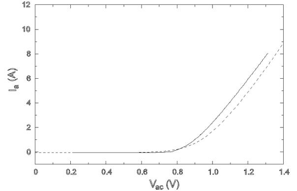
Fig. 14. Comparison between measurement (—) and simulation (- -) of DC-characteristic with extracted parameters.
