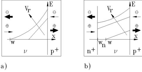
Fig. 3. Electric field in  $p^+\nu^-$  (a) and  $p^+\nu n^+$ -structures (b) at various reverse voltages.
