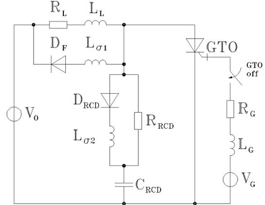
Fig. 4. DC-chopper ( $V_0 = 4\text{kV}$ ,  $V_G = -15\text{V}$ ,  $R_L = 1.33\Omega$ ,  $L_L = 25\mu\text{H}$ ,  $R_{RCD} = 4\Omega$ ,  $C_{RCD} = 6\mu\text{F}$ ,  $R_G = 2\text{m}\Omega$ ,  $L_G = 0.4\mu\text{H}$ ,  $L_{\sigma 1} = L_{\sigma 2} = 0.2\mu\text{H}$ ).
