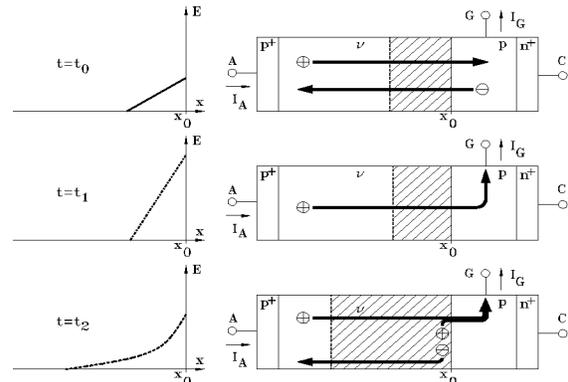
Fig. 5. Dynamic avalanche breakdown in a GTO, carrier flow and field distribution ( $t_0$ : before the onset of avalanche multiplication,  $t_1$ : instable case,  $t_2$ : stable case,  $i_a$ : anode current,  $i_g$ : gate current).
