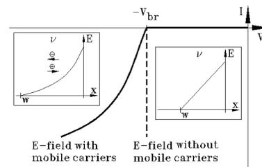
Fig.1. Avalanche generation current in power devices *with* and *without* consideration of generated carriers ( $V_{br}$ : breakdown voltage).
