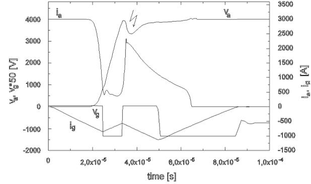
Fig. 8. Dynamic avalanche breakdown of a GTO-thyristor - circuit simulation with SABER. The flash symbol marks the point of maximum power dissipation ( $v_a$ : anode-cathode-voltage,  $v_g$ : gate voltage,  $i_a$ : anode current,  $i_g$ : gate current).
