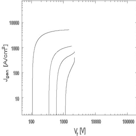
Fig. 6. Post-avalanche behaviour of  $p^+\nu$ -diodes, simulated with eqn. (7).
