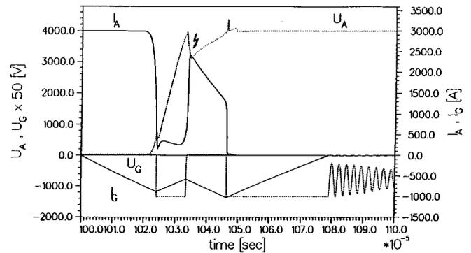
Fig. 9. Dynamic avalanche breakdown of a GTO-thyristor - 1-D device simulation with MEDUSA (taken from Gerstenmaier [6]). The flash symbol marks the point of maximum power dissipation ( $U_A$ : anode-cathode-voltage,  $U_G$ : gate voltage,  $I_A$ : anode current,  $I_G$ : gate current).
