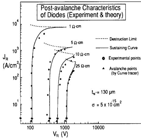
Fig. 7. Post-avalanche behaviour of  $p^+\nu$ -diodes, measured and numerically calculated with basic equations, taken from Takata et al. [5].
