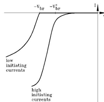
Fig.2. Avalanche current for *low* and *high* initiating currents. Note the decrease of breakdown voltage and the different waveform at high currents ( $V_{br}$ ,  $V_{br}^*$ : breakdown voltages).
