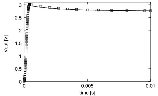
FIGURE 10:  $V_{out}$  OF THE BUCK CONVERTER. — CONVENTIONAL SIMULATION,  $\diamond$  FAST SIMULATION.
