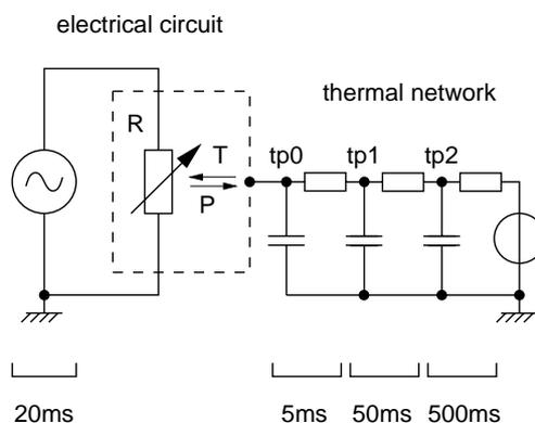
FIGURE 1: CIRCUIT WITH NONLINEAR RESISTOR.
