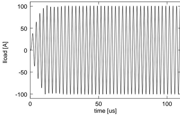
FIGURE 12: CURRENT OF THE LOAD INDUCTOR.
