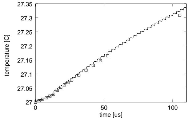
FIGURE 14: CHIP TEMPERATURE OF A MOS-FET. — CONVENTIONAL SIMULATION,  $\diamond$  FAST SIMULATION.
