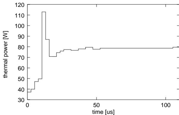
FIGURE 13: AVERAGED DISSIPATED POWER OF A MOS-FET (AVERAGED OVER ONE PERIOD).
