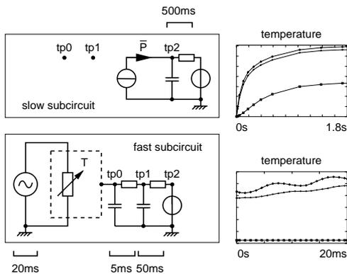
FIGURE 3: PARTITIONING IN SUBCIRCUITS.
