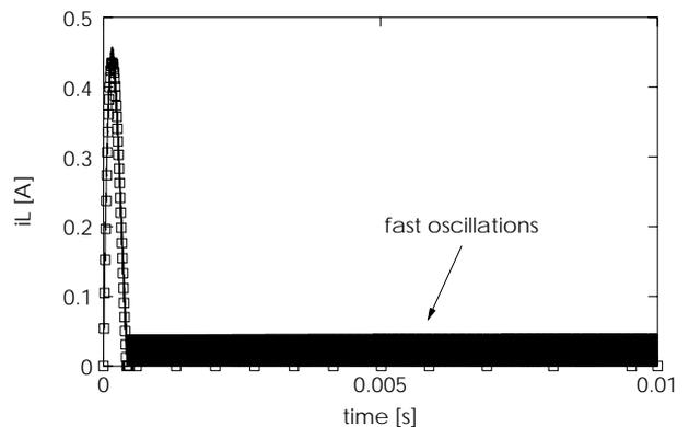
FIGURE 11:  $i_L$  OF THE BUCK CONVERTER. — CONVENTIONAL SIMULATION,  $\diamond$  FAST SIMULATION.
