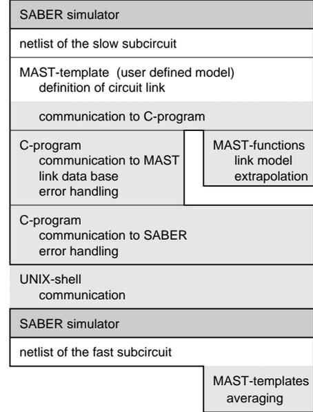
FIGURE 7: IMPLEMENTATION FOR A FAST AND A SLOW SUBCIRCUIT.
