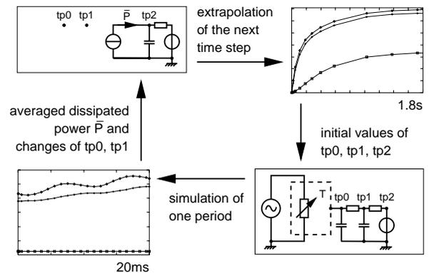
FIGURE 4: LINKING OF SUBCIRCUIT SIMULATION PROCESSES.
